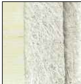
Top fiberglass layer is smooth and strong. Coupled with polyester resin, it resists impact, stains and chemicals.
